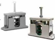
deflection ranges and capacities from 35 to 3,500 lbs (16 to 1588 kg). Alara-Lukagro Model SL and SM spring isolators are typically used to isolate mechanical equipment subject to frequent start-up and shutdown such as compressors and engine generators.
