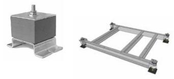
**Equipment Bases | Models CIB and SFB** Custom designed, welded structural steel bases designed to provide rigid support and correct inertia mass providing stability and vibration isolation.
