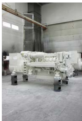
Wet-paint & coating of gensets
