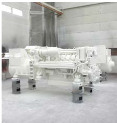
Wet paint and coating of gensets
